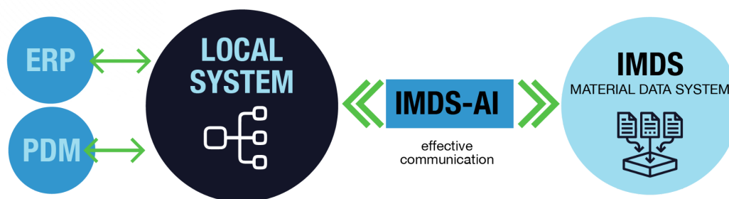
Figure 20 - IMDS system architecture (IMDS, 2022)
